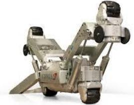
**ULC Gas Pipeline Inspection Robotics**
