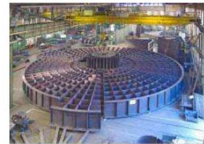
Regenerative preheater – gas/gas
