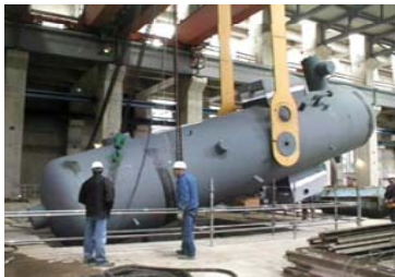
Moisture Separator Reheater
