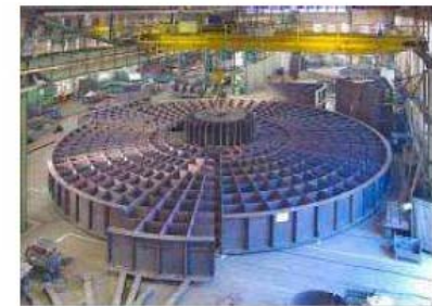
Regenerative preheater – gas/gas
