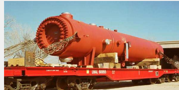
Moisture Separator Reheater
